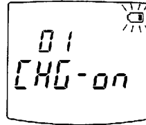
Switching the battery charging "01" On.
